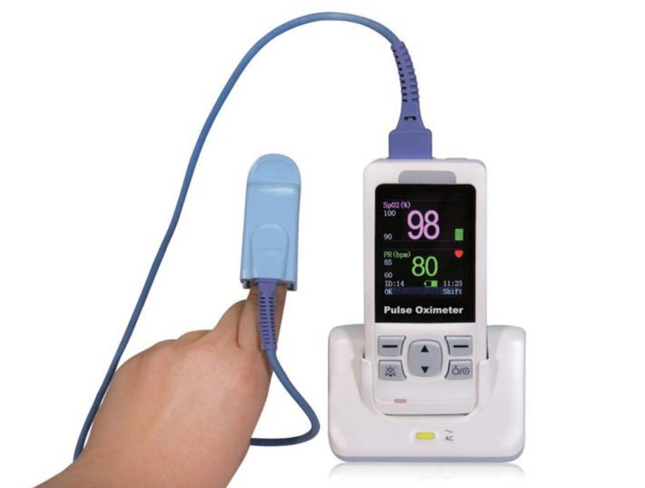
Pulse oximeter is a very important and common device to check patient pulse blood oxygen saturation (SpO<sub>2</sub>) level and pulse rate. As a portable, compact, simple, reliable and durable physiological monitoring device, handheld pulse oximeter AH-MX can greatly enhances patient care. It is widely applied in clinic, hospital, social medical organizations, and first aid and so on.
